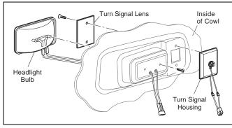
Fig. 18 Headlight and Turn Signal Bulb Replacement
